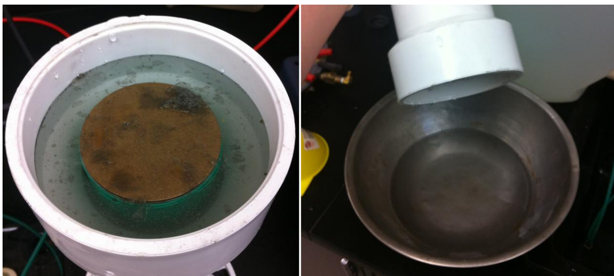
Figure 38: Placement of the porous disk and transferring of the fines lost in the water bath to a container to be oven-dried and weighed.
